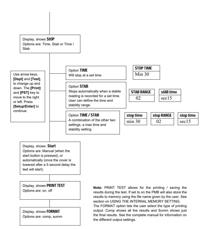
The user can print the current configuration by pressing the **[Print]** key during the process providing the second function for that key is not needed.
